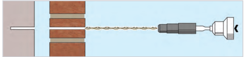
2. Load tie into DryFix Power Driver Attachment fitted to SDS hammer drill
