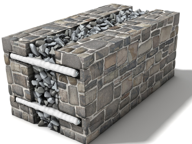
Stabilising a cracked rubble-filled wall.
