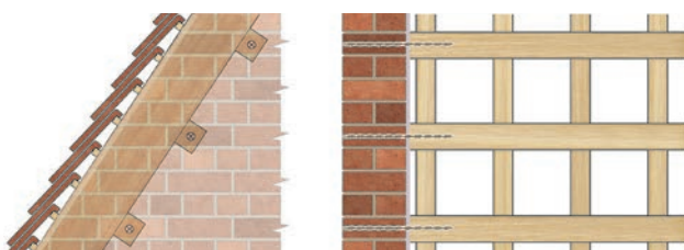
Restraining gable walls using mini retrofit purlins and BowTies
