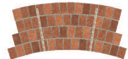
Masonry Arch Pinning of Separated Brick Rings using CemTies
