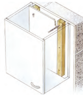
Fixing battens to blocks to support kitchen cupboards
