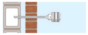
Drill 12mm or 13mm diameter clearance hole in both leaves and flush clean.
