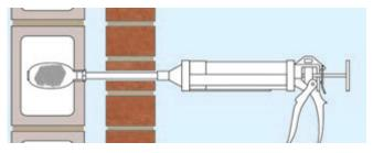
Inject sufficient grout to fill sock and expand it behind far leaf.
