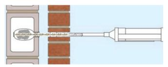
6. Inject grout to fill hole in near leaf and make good.
