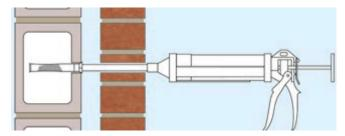
Place sock sleeve over end of grout gun CemenTie nozzle and insert into hole in far leaf.
