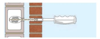
Insert CemenTie, with plastic sleeve fitted, into fabric sock.
