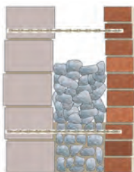
Stabilising bulging rubble-filled wall
