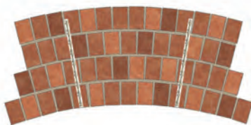
Re-pinning separated brick arch rings
