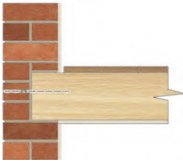
BowTie into joist end through a solid wall
